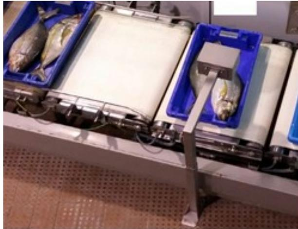
Figure 2- Automatic acquisition unit integrated on a weighing conveyor belt.
